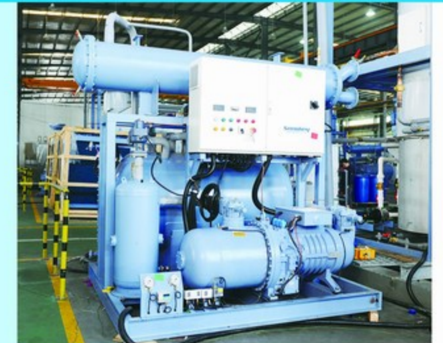
④ compressor condensing unit
